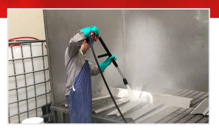
A complete and economical detergent and phosphatizing system for one-step phosphatizing of iron and steel parts. Phosphatizer No. 2 can be used at temperatures ranging from 120°F to 180°F. Equally effective in spray, dip and wipe-on applications. A quality product with 20+ years of successful history in the industry.
